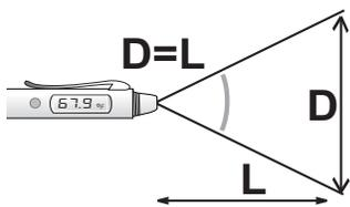
5. Once the button is released, the last measurement will be shown and held until the button is pressed again or until the SIL2 turns off.
